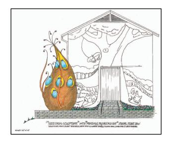
The pedestal to the left will hold a 250-gallon plastic water tank within a large sculpted seedpod form. Created from colored concrete over a metal framework, this rainwater harvesting sculpture will collect water runoff from the roof to be employed both to water the garden and support a water feature (water running down the seed pod into a small pool below) driven by a solar-powered circulating
